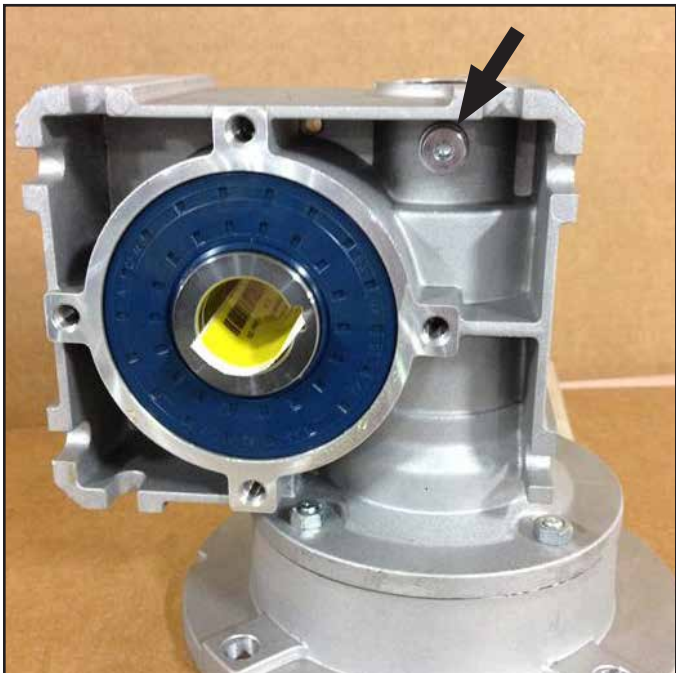
Figure 9-7: Gearbox Oil Fill Valve
