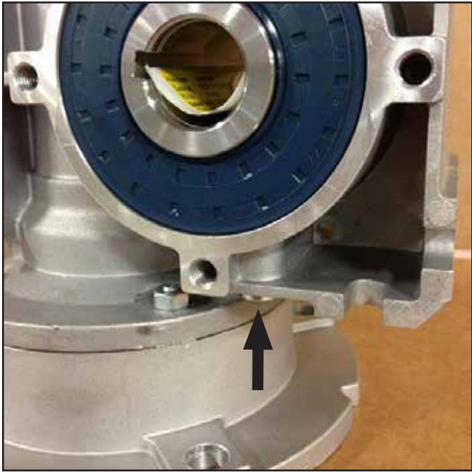
Figure 9-6: Gearbox Oil Drain Valve
