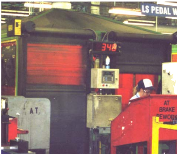
Dual-Guardians allow robotic welding to occur on one side of the cell, while an employee safely loads parts on the opposite side of the cell.
