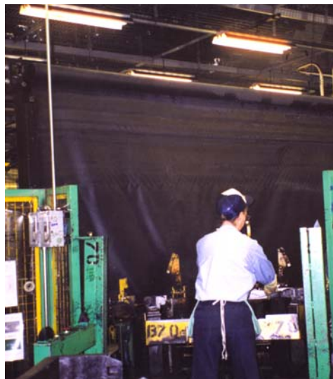
13' wide Guardian helps provide safety from arc flash and prevents entry into the robotic welding cell.
